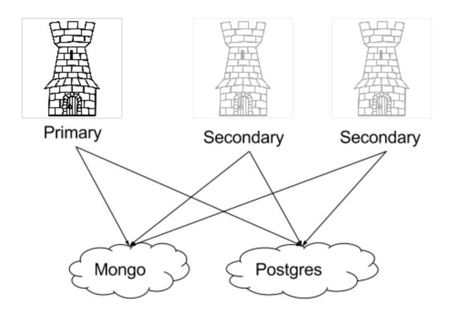
Tower's redundancy offers a standby Tower infrastructure that can become active in case of infrastructure failure—avoiding single points of failure. Redundancy is not meant to run in an active/active or multi-master mode, and is not a mechanism for horizontally scaling the Tower service. Remember that failover to a secondary instance is not automatic and must be user triggered.
