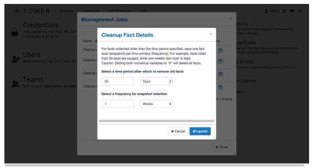
Select the time period after which you want to remove old data as well as the frequency for snapshot retention.
