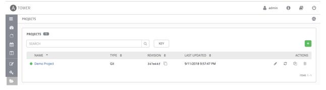
Ansible Tower simplifies the getting started process by providing you with a Demo Project to work with initially.
