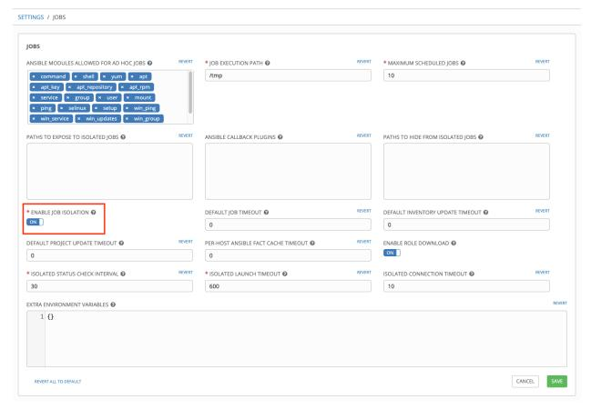
By default, the Tower will use the system's tmp directory (/tmp by default) as its staging area. This can be changed in the **Job Execution Path** field of the Configure tower screen, or by updating the following entry in the settings file:
