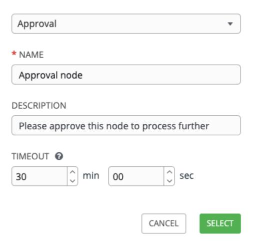
The default for the timeout is none, but you can specify the length of time before the request expires and automatically gets denied. After selecting and supplying the information for the approval node, it displays on the graphical view
