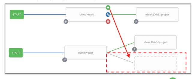
You can insert another node in between nodes by hovering over the line that connects the two until the VV appears.
