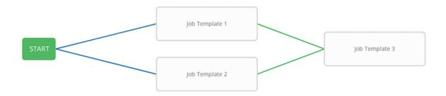
In the example provided, Tower runs the first two job templates in parallel. When they both finish and succeed as specified, the 3rd downstream (*convergence node*), will trigger.
