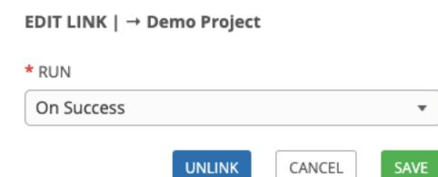
This button only appears in the right hand panel if the target or child node has more than one parent. All nodes must be linked to at least one other node at all times so you must create a new link before removing an old one.
