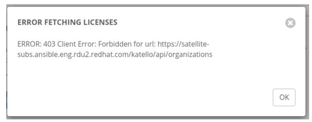
The Satellite username/password is used to query the Satellite API for existing subscriptions. From the Satellite API, the automation controller gets back some metadata about those subscriptions, then filter through to find valid subscriptions that you could apply, which are then displayed as valid subscription options in the UI.
